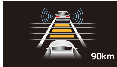
CACC: Cooperative Adaptive Cruise Control: Adjustment of the distance between cars using information provided by the preceding car
